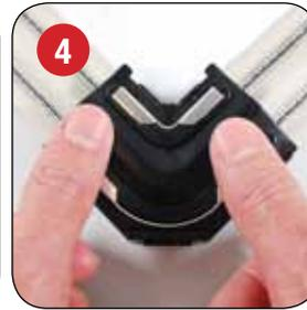
4 Insert the hook-tab on the top under the bar on the outer corner of the bottom part. Then firmly press down so that all four tabs lock in place.
