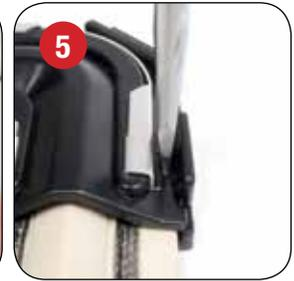
5 To open the part insert a flat screwdriver as shown and gently twist the tabs away from the part. Prying two tabs on the same side is generally all that is needed to remove the top.
