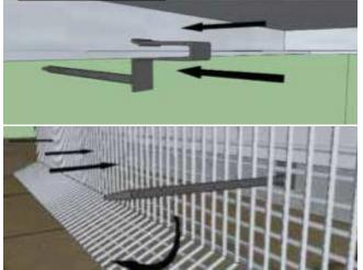
STEP 1: Place clips every 18 inches. Slide the clip onto the edge of the panel support bracket. Slide as far outward as possible so the clip is all the way on the lip of the panel.
